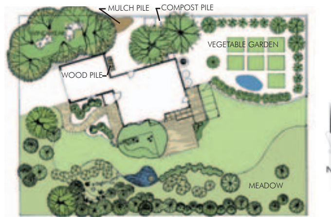
This plan view illustrates how a home can be oriented to the south to maximize southern exposure for day lighting and solar access. As well, this plan combines other elements of a sustainable landscape.
