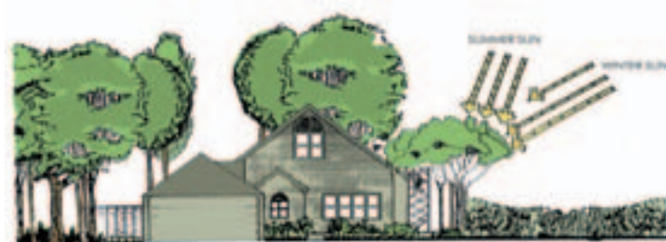
During winter, the sun reaches far inside the house, due to its low angle. The deciduous trees are leafless, allowing approximately 50% of the sun's rays through to heat the house. During summer, up to 96% of the hot summer sun's direct rays are blocked by deciduous trees planted around the south-southwest sides of the house keeping the house cool during the hot summer months.
